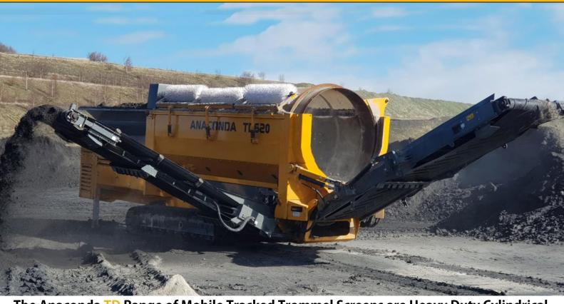
The Anaconda TD Range of Mobile Tracked Trommel Screens are Heavy Duty Cylindrical Screens that has been designed specifically for exceptional results in testing scenario's.
