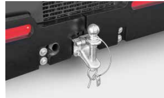
Trailer Hitch Homologated for use in road transit 115990101
